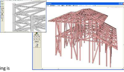
As external forces, STAN/3D is able to treat nodal load and member load, enforced displacement, temperature load, and self-weight, and combinations of these can also be analyzed. STAN/3D can also be used in analyses that consider factors such as settings for compression members and tension members and the uplift of the foundations, enabling the reflection of boundary (constraint) conditions and a variety of other considerations introduced by multiple designers.
